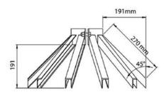
D - A one-way anti-climbing device fixed 2.65M high (under the inspection chamber) has a dual function: it prevents malicious persons from climbing and reach the inspection chamber and allows joining mast and shells.
