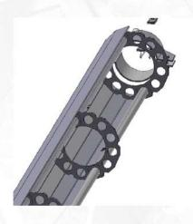
B - A patented external device made of two half shells, each one is fitted with 6 specific, removable and tubes. These two half-shells replaceable assembled to form an external envelope around the entire periphery of the mast in order to protect it from attacks by a battery-powered disk grinder. This is achieved by delaying, blocking or expelling the malicious grinder disc.
