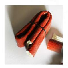
C - A fireproof sheath, Ø38mm made of natural fibre runs through the mast centre.
